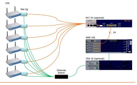
It is possible to expand the DMS, which makes the DMS very suitable for large volume production testing. CDE
